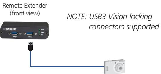
Figure QS-5. Connect the USB device to the Remote Extender.
