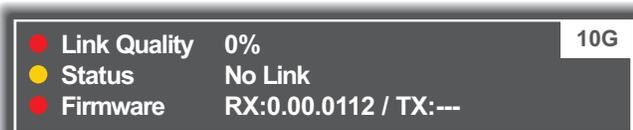
The color of the Dashboard's **Link Quality** indicator matches the front panel **LNK** indicator:
